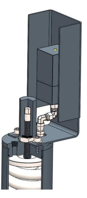
Figure 2. PN 29094 1" Gen 2 Pressure Regulator, Manual Spring, Detailed sealed spring chamber.
