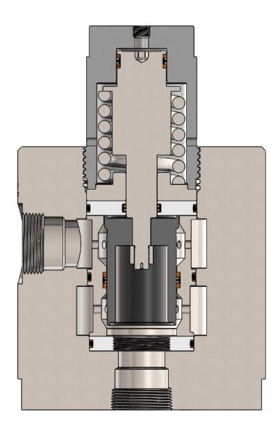
Gilmore has met or exceeded API 16D requirements by qualifying the new 1-1/2 inch GEN2 SPM designs to multiple endurance qualification tests to 2500 cycles, at 5000 psi and 250 GPM, with 1% - 4% water glycol test fluid.
